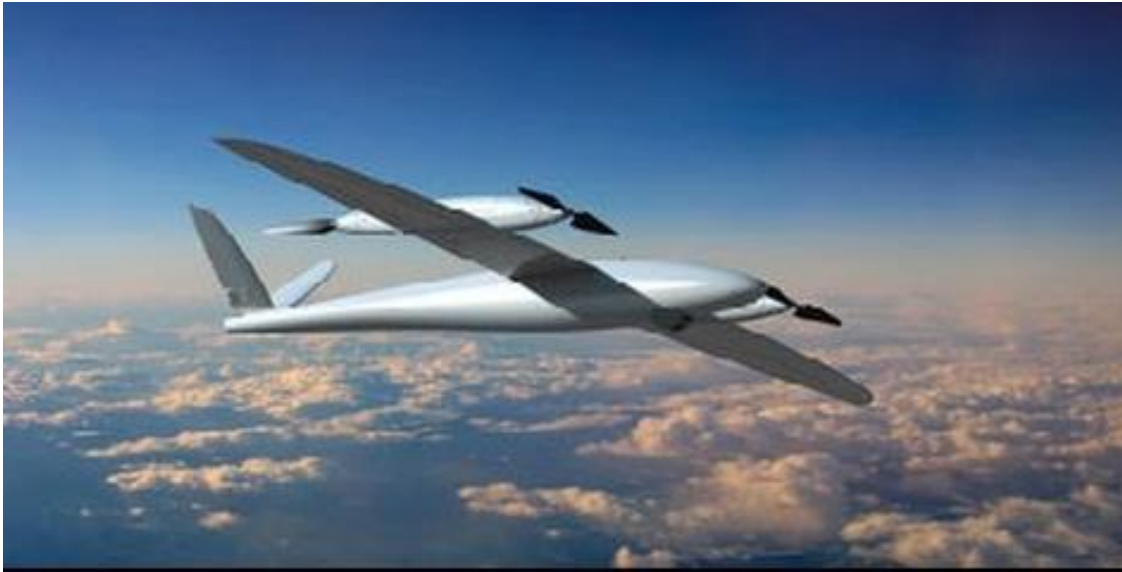
Figure 5-5: H1 Tron – Fuel Cell Electric Hybrid Fixed wing VTOL
