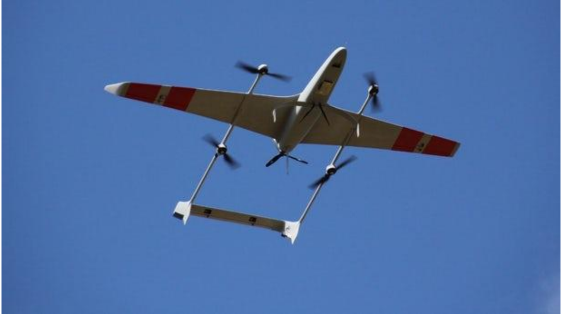
Figure 5-3: Volanti Hybrid (Electric / Gasoline) Fixed Wing VTOL Aircraft
