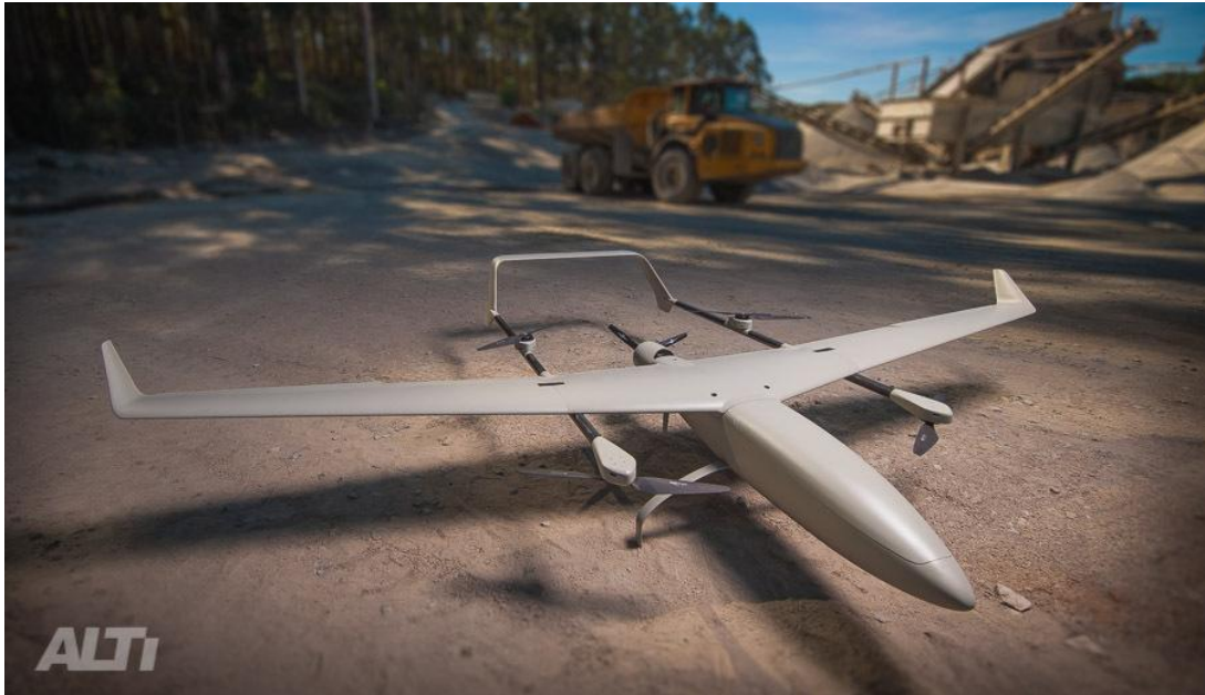
Figure 5-4: ALTi Transition (Electric / Gasoline) Fixed Wing VTOL UAV
